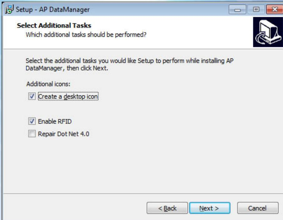
To install Data Manager, run **setup.exe** from the installation CD. Be sure to check the **ENABLE RFID** box.
