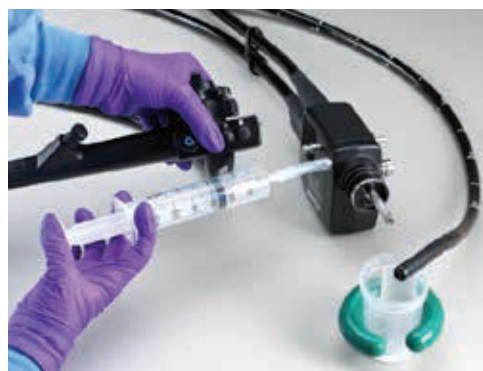
Sampling a Fujinon® flexible endoscope
