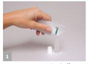
Open Type 8 extraction buffer sachet and add to a sample tube.
