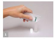
Open Type 8 extraction buffer sachet and add to a sample tube.
