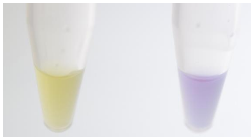
Picture 1. Typical appearance of a positive fermentation reaction (left) and a negative reaction (right)
