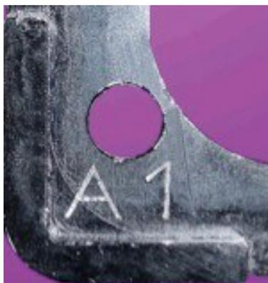
Figure 20. Bottom left-hand corner of plate carrier illustrating the 'A1' mark
