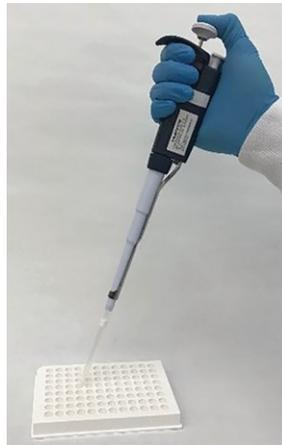
Figure 19. Pipette the sample into the bottom of the wells
