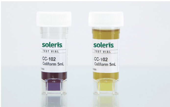
CC-102 Vial uninoculated (left) and inoculated vial (right).
